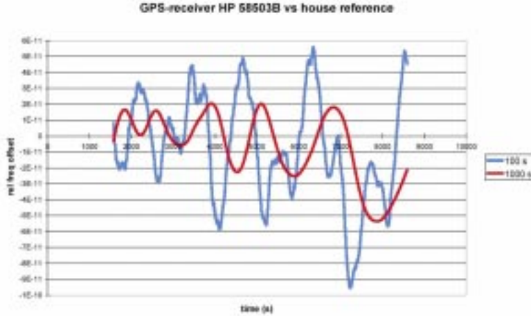
Figure 4: Frequency variation of a GPS-disciplined OCXO over an observation period of some hours. The average output frequency over 100s intervals varies from -1*10^{-10} till +6*10^{-11} . Measurements performed at Pendulum Instruments AB
