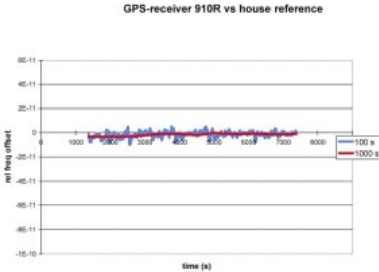
Figure 5: Frequency variation of a GPS-disciplined Rubidium oscillator over an observation period of some hours. The average output frequency over 100s intervals varies from -9*10^{-12} till +4*10^{-12} . Measurements performed at Pendulum Instruments AB
